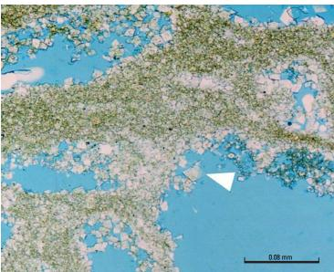
Note partial dissolution of dolomite rhombs (white arrow) to form larger pore spaces Sample impregnated with blue-dyed epoxy to highlight pore space
