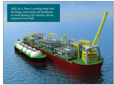
The broad operating parameters of the Shell design mean it can be redeployed, said Shell. Its standardized "design one—build many" approach permits "material repeatability gains" during design and construction. After completing the FEED phase, Shell said it will examine key aspects of each potential FLNG project in its portfolio before considering a final investment decision.
