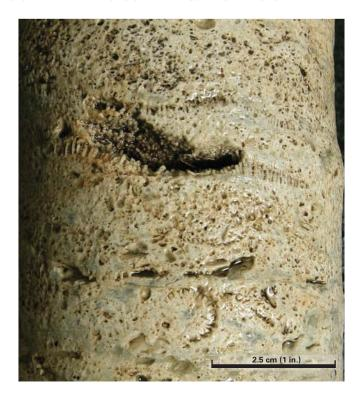
characterized by interbedded limestone, dolomite, silty argillaceous dolomitic limestone or dolomite, and calcareous shale.
